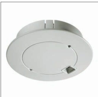
Light sensor intended for high-bay mounting (approx. 7.5 m high). Intended for use with the Linesense control (ZTX400 MDU-D). An installation bracket is included. The sensor is connected to the control unit with a modular plug-in (RJ-12) connector cable
